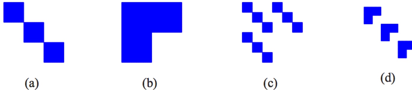
Figure 1: Examples of network block models. (a) Community structure, (b) core-periphery structure, (c) global core-periphery structure with local community structure, and (d) global community structure with local core-periphery structure. Note that (c) and (d) are equivalent.
